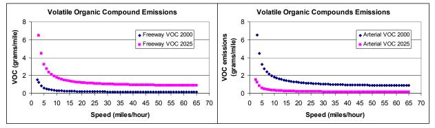
In addition to these "steady speed" emission rate values, emissions tend to be highest during acceleration. Engine operation is less efficient during these times and more unburned fuel is sent through the exhaust system.
